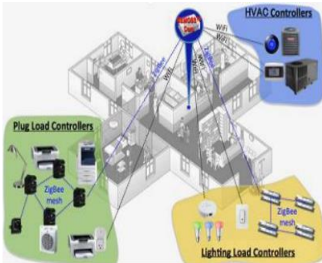
Fig. 1. BEMOSS system architecture for commercial buildings
